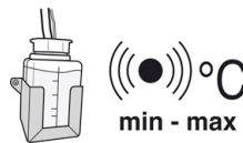
Ballasted sensor for simulation of product temperature alarm
